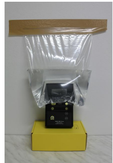
Cesium-137 measurement of foodstuff Accuracy \pm 200 Bq/l
