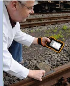
A wide Pulse Repetition Frequency range. This allows the USM Go to be used at low PRF to inspect forged parts for inclusions and porosity without any "ghost" echoes and just as easily find application in weld inspection at high PRF when fast and regular scanning movement is required to optimize inspection times.
