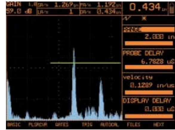
Four digital reading boxes at top display trigonometric calculations for weld inspection (SA soundpath to flaw in gate A, PA projection distance to flaw in gate A, DA depth to flaw in Gate A & LA leg of inspection that flaw occurs in gate A)
